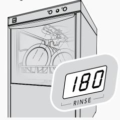
Wash cycle is extended if the final rinse temperature is not maintained at 180°F/82°C. Machine will begin Heat Recovery cycle after rinse cycle.
