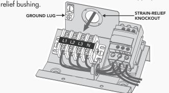
You must leave 30" of wire to allow the machine to be pulled from it's installed position for servicing.
